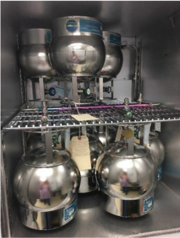
Figure 29. Laboratory canister cleaning setup.
