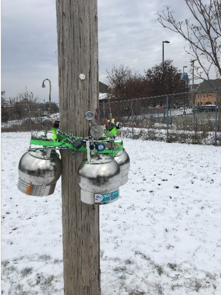
Figure 20. Example of EtO ambient sampling set up.
