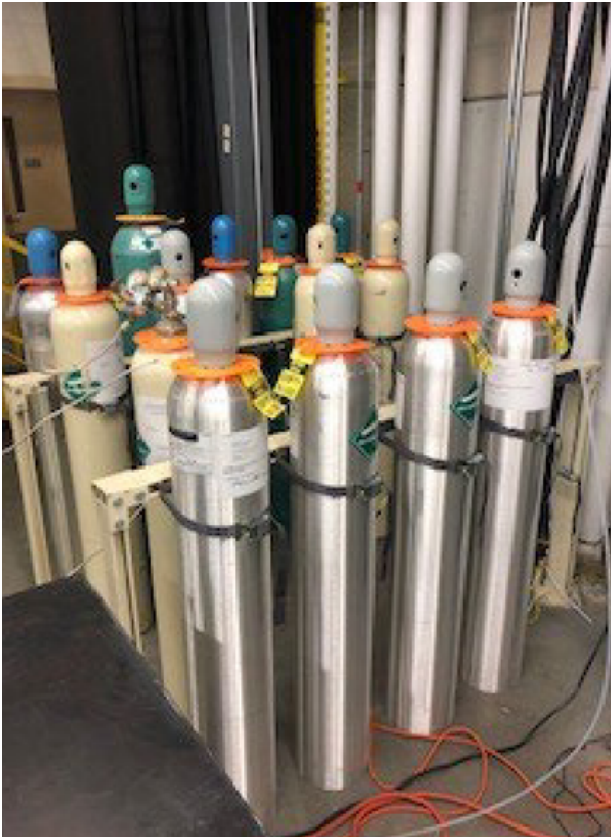
Figure 27. Cylinder gases used to calibrate analytical equipment.
