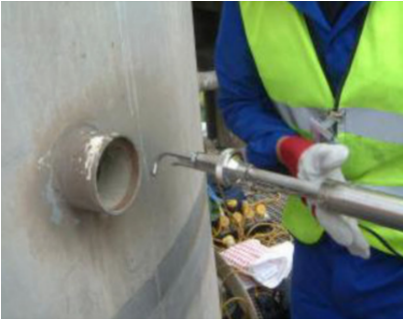
Figure 25. Sampling probe being removed from an emissions stream.
